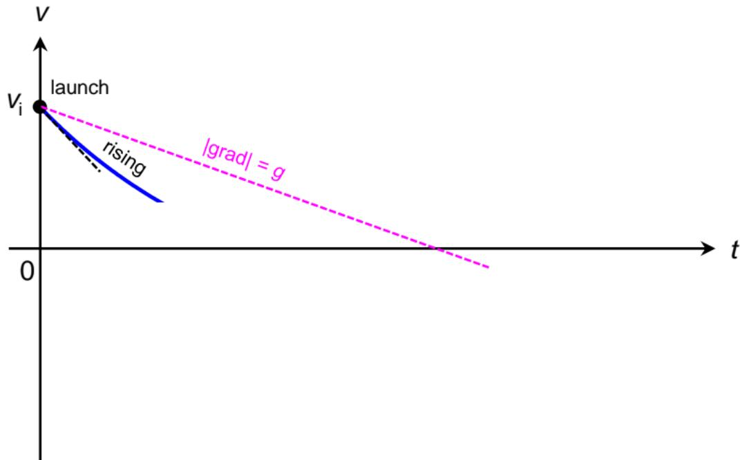
Remember that drag force is dependent on speed. As the balloon loses speed,  $R$  decreases. As  $mg+R$  decreases, the speed drops towards 0 at decreasing rate.
