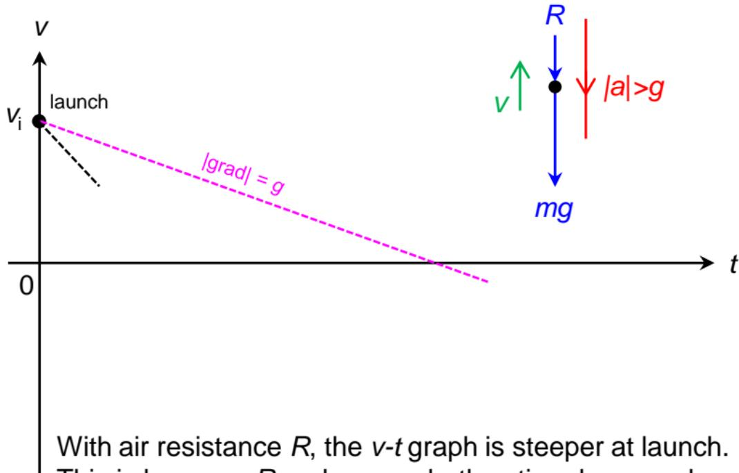
With air resistance  $R$ , the  $v$ - $t$  graph is steeper at launch. This is because  $R$  and  $mg$  are both acting downward, combining to make  $mg+R$  total retardation force, resulting in the balloon slow downing at a rate higher than  $9.81 \text{ m s}^{-2}$ .
