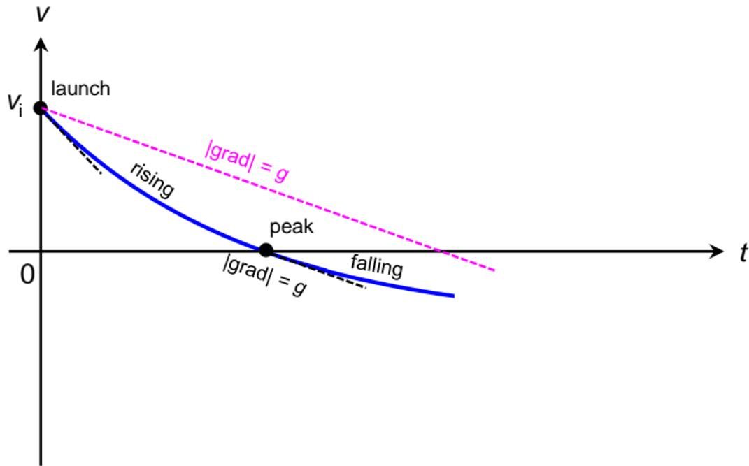
Remember that drag force is dependent on speed. As the balloon gains speed,  $R$  increase. As  $mg - R$  decreases, the balloon gains speed at decreasing rate.
