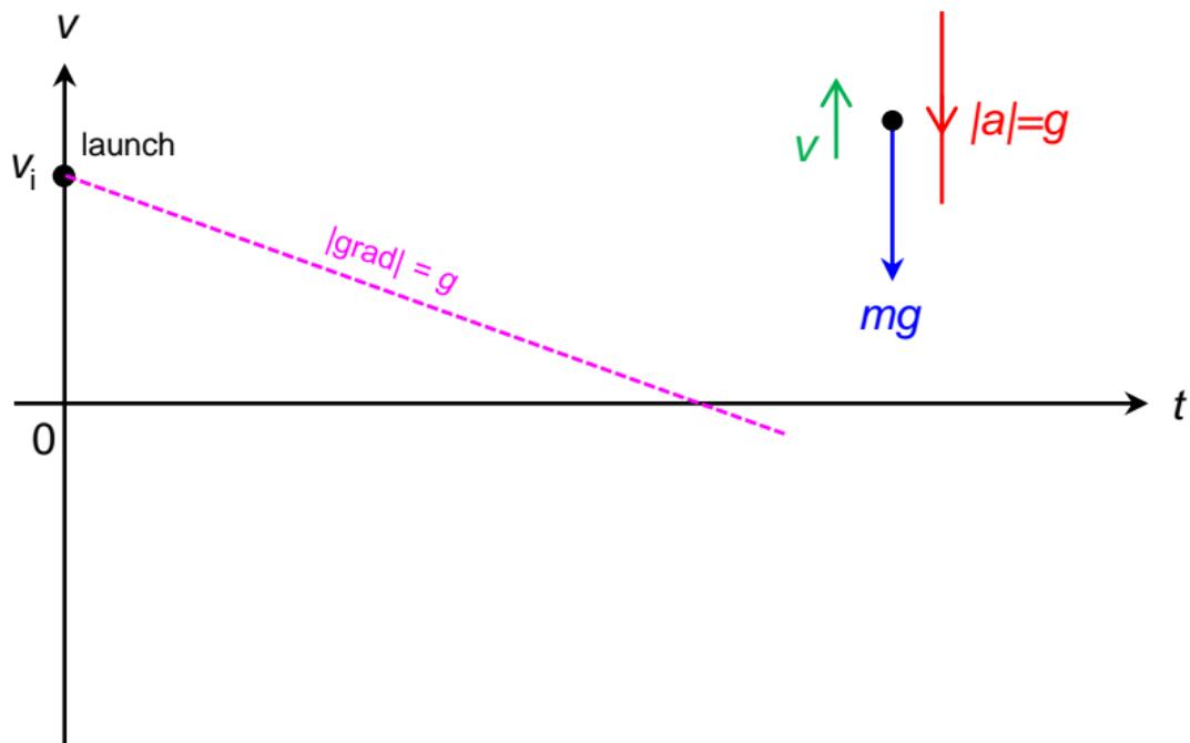
If there were no air resistance, the balloon would be slowing down at constant rate of  $9.81 \text{ m s}^{-2}$ . And the  $v-t$  graph would be the magenta line.
