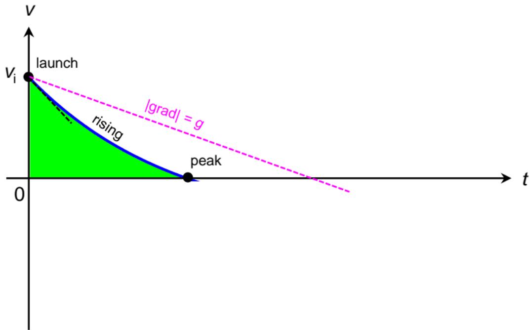
The green area corresponds to the upward distance travelled by the balloon.
