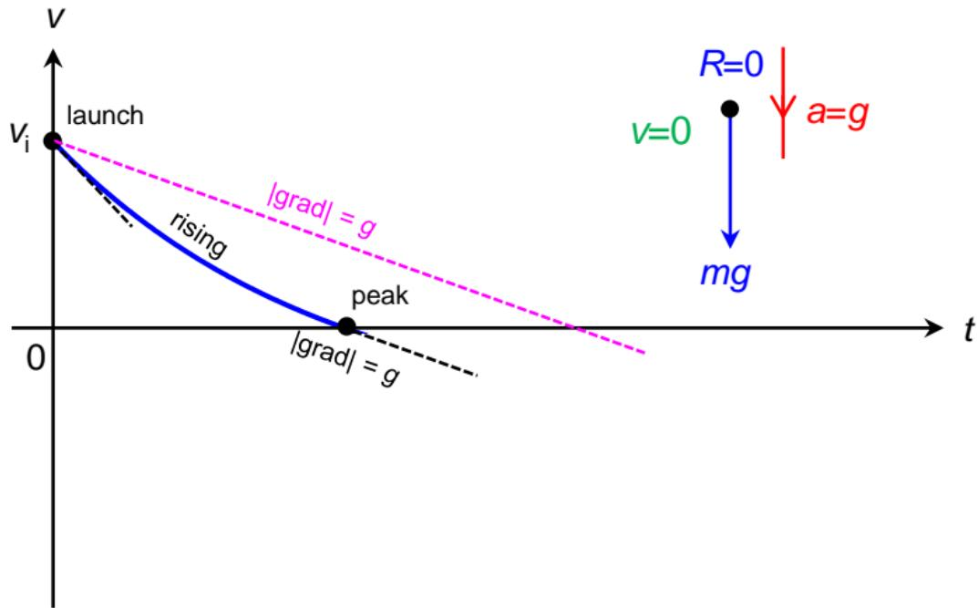
Since  $R$  is zero when  $v=0$ , the gradient at this instant is  $9.81 \text{ m s}^{-2}$ .
