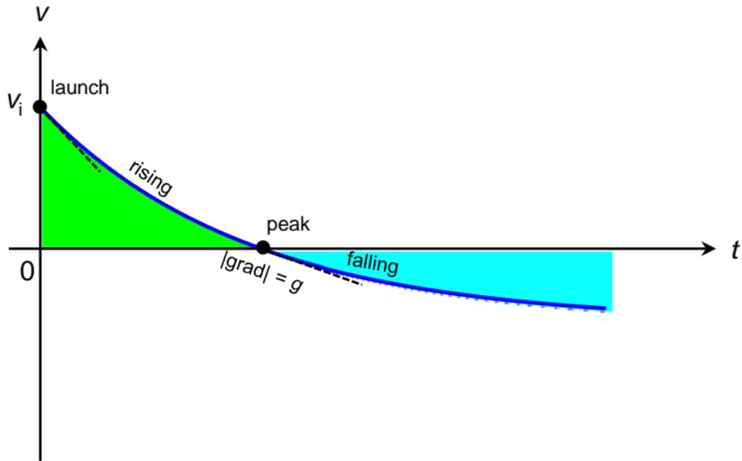
The graph ends when the blue area matches the green area, when the downward distance matches the upward distance.
