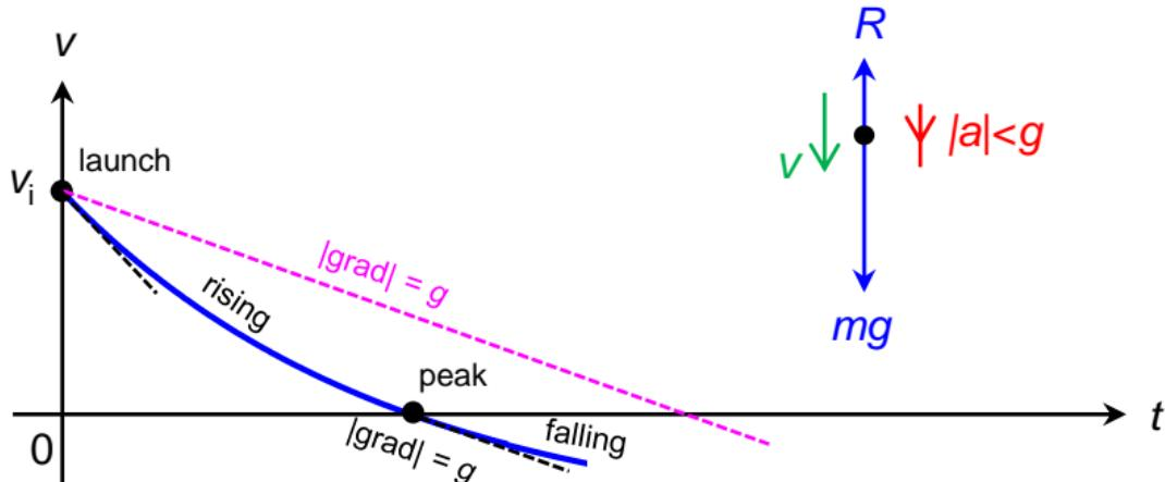
During the descent, the graph becomes even less steep. This is because  $R$  is now acting upward in opposite direction to  $mg$ , reducing the net force to  $mg - R$ , resulting in the balloon speeding up at a rate lower than  $9.81 \text{ m s}^{-2}$ .
